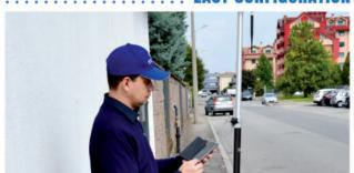
Connect your mobile phone to the receiver Wi-Fi to change settings and monitor the receiver status using a standard web browser.
