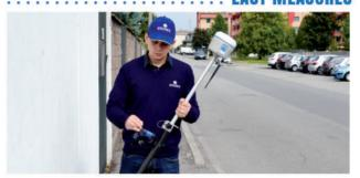
It's very easy to measure corners or edges of walls. Internal sensors can correct the coordinates of the points collected according to the tilt angle and tilt direction.
