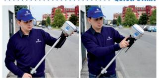
By a quick press, users can easily insert and remove \$10 from the range pole.
